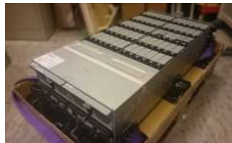
Figure 22: Vendor's early-engineering sample of a high-density-high-performance storage system being unwrapped at the Nikhef Data Processing Facility.
