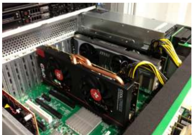
Figure 23: Experimental system at the Nikhef Data Processing Facility for general-purpose GPU (vector-processing) programming, comparing GPU architectures and their science application performance.
